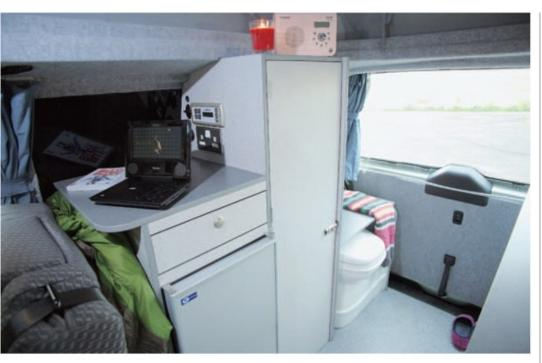
fridges not only save on gas usage but also have other benefits such as the ability to work on sharper gradients, are more efficient in reaching their working temperature, and you don't have to remember to change their power source manually. The only disadvantage is that I decided to sleep on the offside bed – the fridge was just behind my pillow and the noise of it switching on and off to maintain its temperature did wake me up once or twice.
