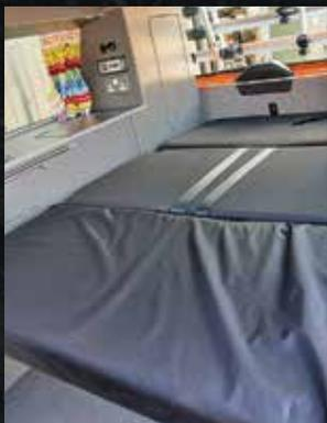
The T3ree as tested is part of Jerba's small hire fleet hence the seat covers fitted while in use. The cab seats swivel to allow for four to sit around a table that packs away behind the driver's seat.
