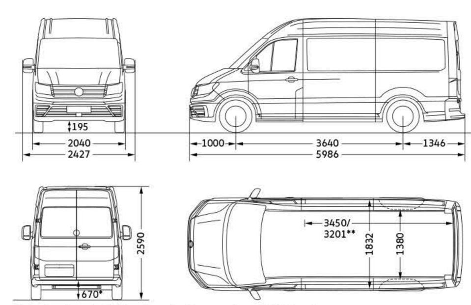
Illustration shown is CR35 medium wheelbase panel van with high roof.
