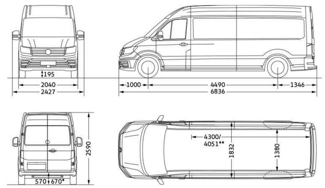
Illustration shown is CR35 long wheelbase panel van with high roof.
