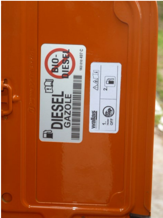
Warning labels applied to fuel filler flap.
