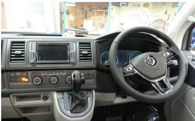
Warning lamp which shows when the space heater is on.
