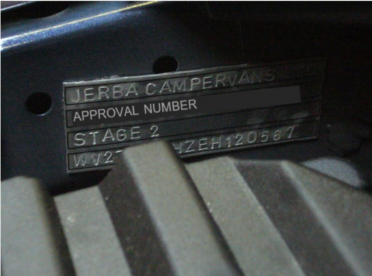
Position of plate on vehicle under bonnet all versions.
